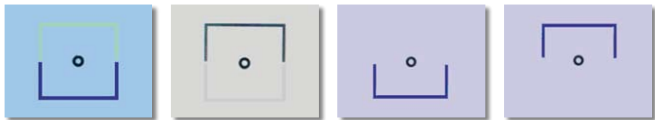
Ghost images and different background colors in conventional LCD chart systems
